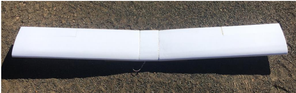
Figure 2 - Removable wing using Clark Y airfoil
